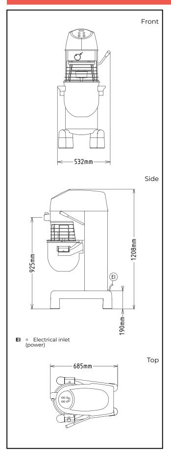
Electric Supply voltage: 200-240 V/1N ph/50/60 Hz **Electrical power max:** 1.1 kW **Total Watts:** 1.1 kW Capacity: Performance (up to): 7 kg/Cycle Capacity: 30 litres Key Information: External dimensions, Width: 532 mm External dimensions, 685 mm Depth: External dimensions, Height: 1208 mm **Shipping weight:** 114 kg **Cold water paste:** 7 kg with Spiral hook 50 with Whisk Egg whites:
